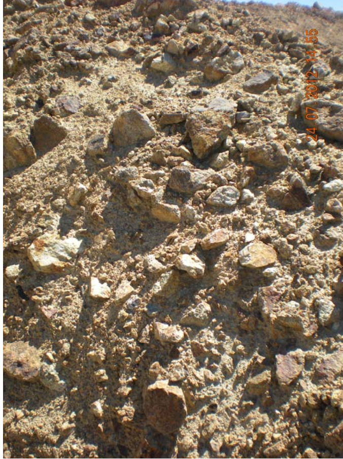
Photo 1. Matrix dominated rockfill observed in 2012.
